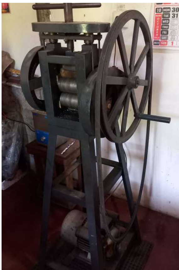
Hand-powered machine for silver rolling
